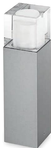
Lighting fixtures for floor mounting. Integrated compact fluorescent lamp or LED light source. Antioxidant polyester powder-coated extruded aluminium casing. Lead glass diffuser.
