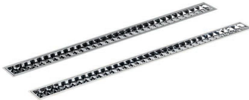
Recessed lighting fixtures for false ceiling or brick mounting by means of recessed housings. Anodised or coated extruded aluminium profile. High performance, low luminance specular aluminium dark light diffuser, with fluorescent linear light source.
