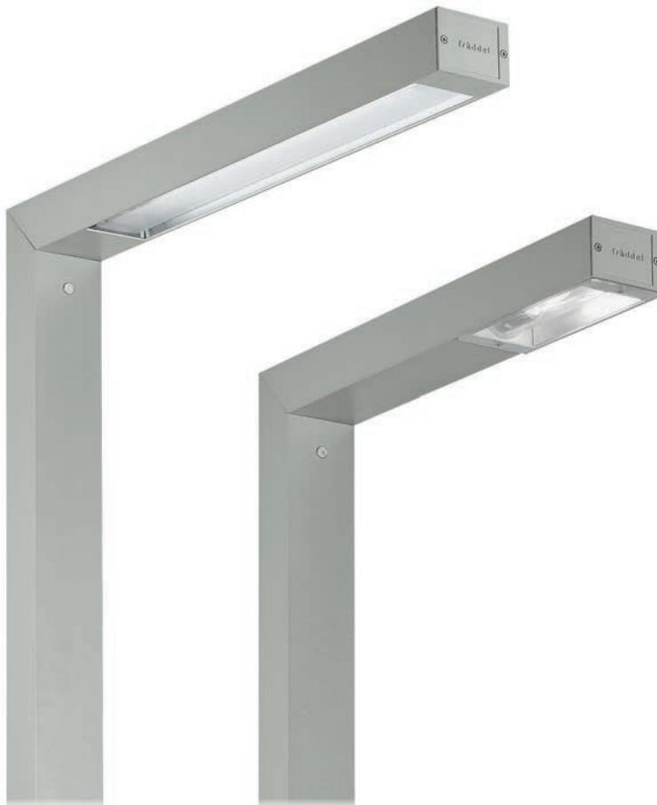
Direct light lighting system with variable section post. Upper structure made of high chemical resistant polyester powder-coated extruded aluminium. Lower section made from coated galvanised steel tubing. Light source consisting of fluorescent lamp and multi-power supply unit, or of gas discharge lamps. Transparent grooved polycarbonate diffuser with high light efficiency. "Cut-off" emission with no flux emitted upwards. Versions with or without double switch-on point auxiliary LED lighting.
