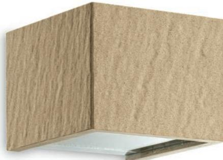
Double emission lighting fixture for wall mounting. Halogen or LED light source with integrated driver. Quartz composite stone casing with hard anodised aluminium internal structure. Polished AISI 316 stainless steel brackets and toughened glass diffuser.
