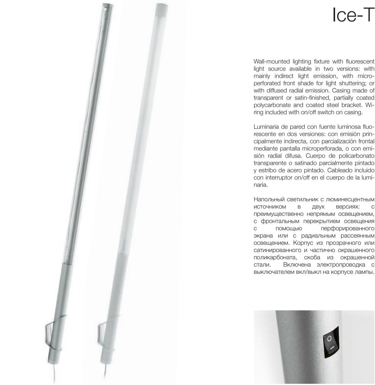
Wall-mounted lighting fixture with fluorescent light source available in two versions: with mainly indirect light emission, with micro-perforated front shade for light shuttering; or with diffused radial emission. Casing made of transparent or satin-finished, partially coated polycarbonate and coated steel bracket. Wiring included with on/off switch on casing.
