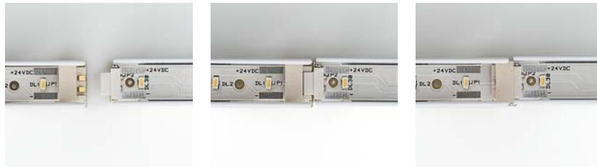
Put plug connector closer to socket connector.
