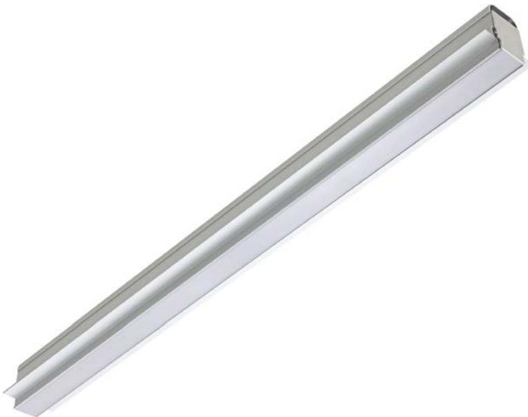
Trimless recessed lighting fixture provided with through wiring and fitted with highly-efficient SMD LED light source, or a linear fluorescent lamp. It can be installed on partitions and false ceilings. Anodised extruded aluminium profile. Opal polycarbonate diffuser. Driver included.
