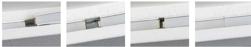
LED sources on rigid circuit housed in dissipating extruded aluminium and fitted with a protective diffuser made of polycarbonate. Quick connection system between lighting elements on EPS profiles through magnetic contact. Elements with 500mm standard length can be cut every 100mm.
