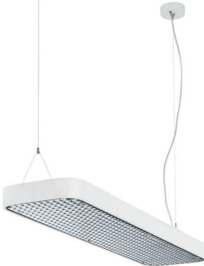
Double emission suspension light with fluorescent light source. Shaped and coated extruded aluminium casing. Dark light diffuser with special front silk-screened pattern. The ceiling rose can be mounted in line with a supporting cable or decentralised.
