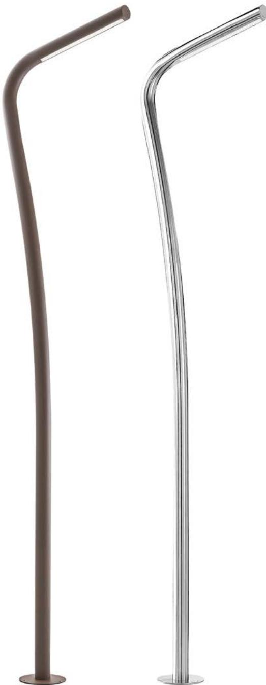
Floor-mounted lighting fixture with post integrated base and peg or anti-vandal bracket with log bolts. High brightness SMD LED light source protected by a satin-finished diffuser to enhance light distribution.
