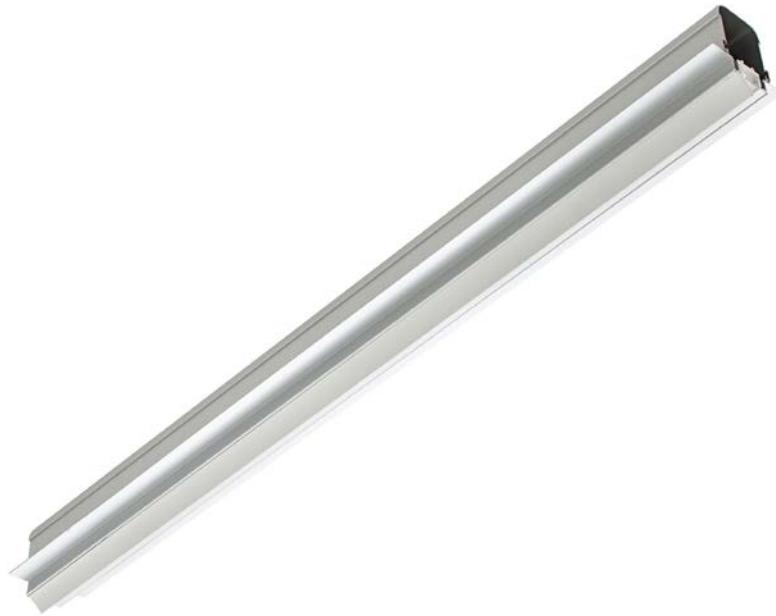
Trimless recessed linear module designed to create continuous lines of light with asymmetric emission. It can be mounted on false ceilings. The lighting fixture is provided with through wiring and fitted with a highly-efficient SMD LED light source. Anodised extruded aluminium profile. Opal polycarbonate diffuser. Driver included.
