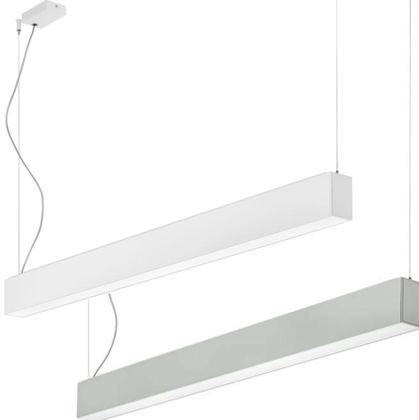
Single emission lighting fixture for suspension mounting with fluorescent light source, or with double emission in hybrid version, with fluorescence and LEDs, or with only LEDs. Anodised or coated extruded aluminium profile fitted with end caps. Opal PMMA diffuser. Double emission articles are designed for a double switch-on point.
