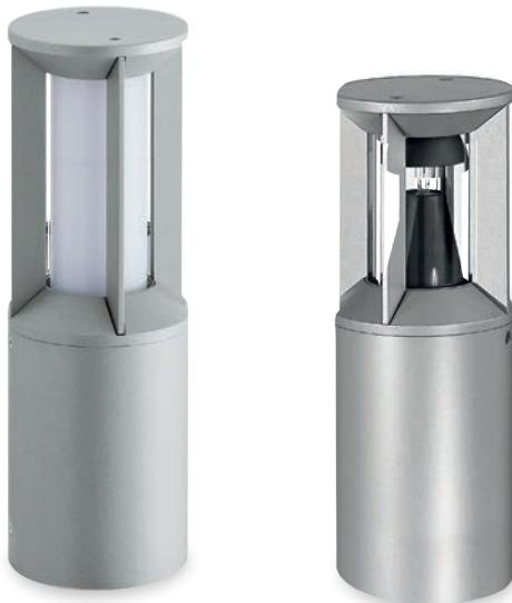
Ground-mounted lighting fixture available in the versions for direct downward lighting with gas discharge source or for diffused lighting with integrated compact fluorescent lamp. Gas discharge lamp version with ballast included.
