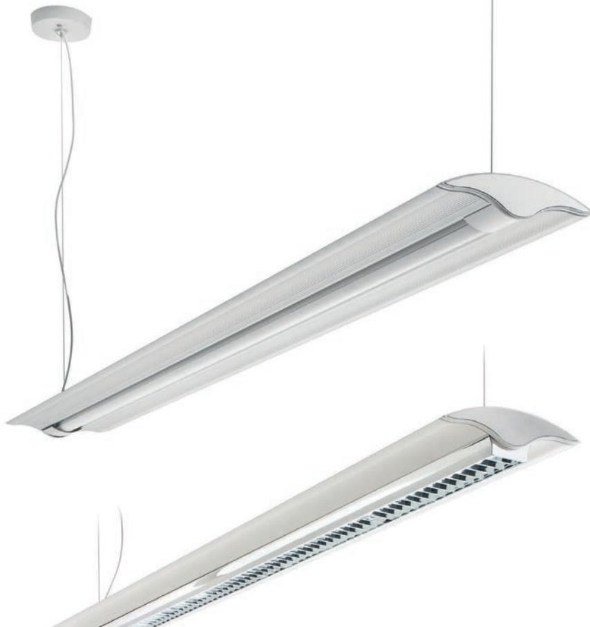
Suspension light to be fitted only with double emission LED tubes. Internal driver. Anodised or coated extruded aluminium casing fitted with end caps, suspension and power supply kits. Available with exposed light source or dark light pure aluminium diffuser for luminance control.
