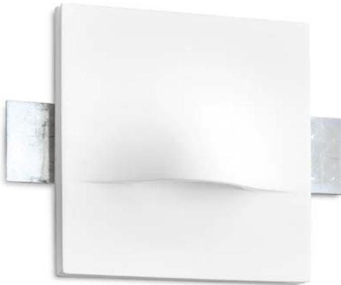
Plaster semi-recessed lighting fixture with fixed optical compartment. LED light source for direct downlighting. Driver not included. It must be installed upline in the connector box.
