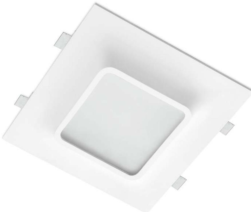
Plaster semi-recessed lighting fixture fitted with satin-finished polycarbonate diffuser. It can be installed on 600 x 600 modular false ceilings or on standard false ceilings. Fluorescent light source. Electronic ballast included.
