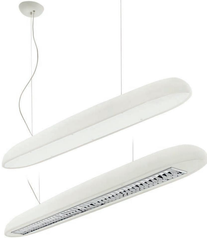
Suspension light with linear T16 seamless fluorescent lamps. Natural polyethylene casing for diffused light emission. It is fitted with microprismatic PMMA diffuser or with louvered optics integrated in an opal PMMA diffuser.
