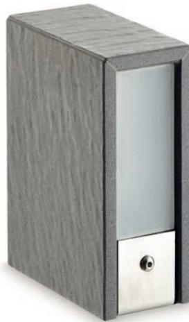
Single emission lighting fixture for floor mounting. LED light source with integrated driver. Quartz composite stone casing with hard anodised aluminium internal structure. Polished AISI 316 stainless steel brackets and sandblasted toughened glass diffuser.
