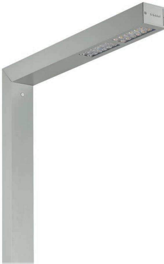
Direct light lighting system with variable section post. Upper structure made of high chemical resistant polyester powder-coated extruded aluminium. Lower section made from coated galvanised steel tubing. LED light source and "cut-off" emission with no flux emitted upwards.
