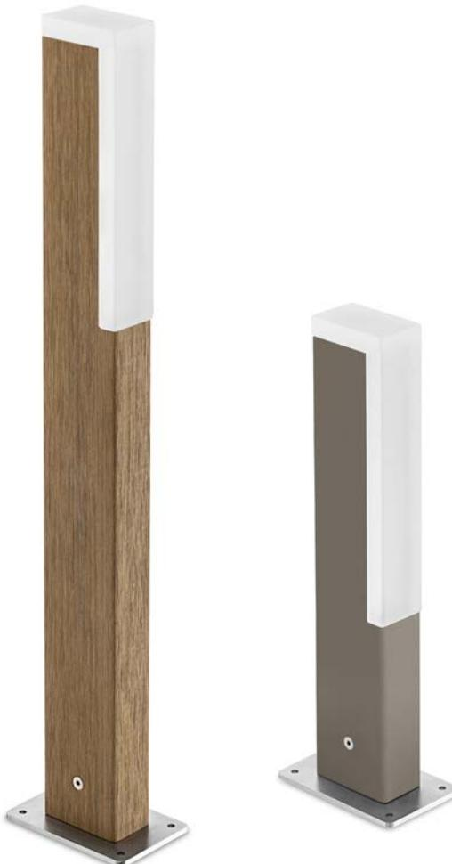
Lighting fixture for ground mounting with diffused light emission. Technical wood casing with grained or smooth surface in the oak or aluminium grey colour version respectively. The fixing elements are made of stainless steel while the diffuser is made of polymethylmethacrylate. LED strip light source.
