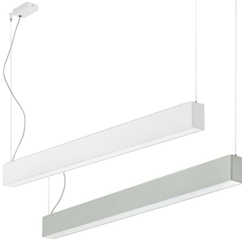
Single emission lighting fixture for suspension mounting with fluorescent light source, or with double emission in hybrid version, with fluorescence and LEDs. Anodised or coated extruded aluminium profile fitted with end caps. Anti-glare microprismatic PMMA diffuser. Double emission articles are designed for a double switch-on point.
