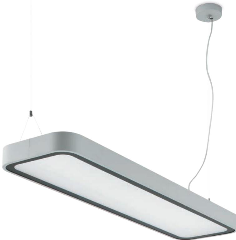
Double emission suspension light with LED light source. Shaped and coated extruded aluminium casing. Microprismatic PMMA diffuser. The ceiling rose can be mounted in line with a supporting cable or decentralised.
