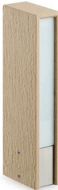
Double emission lighting fixture for floor mounting. Linear or compact fluorescent light source with integrated ballast. Quartz composite stone casing with hard anodised aluminium internal structure. Stainless steel brackets and silk-screened and sandblasted toughened glass diffuser.
