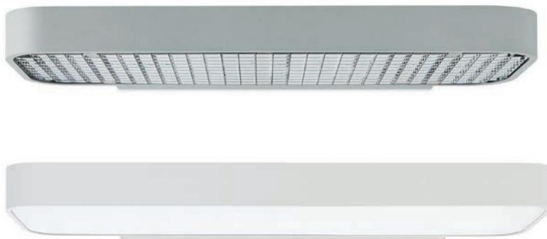
Double emission wall light with fluorescent light source. Shaped and coated extruded aluminium casing. Available with dark light or microprismatic PMMA diffuser for a balanced luminance control or with anti-glare opal polycarbonate diffuser for even distribution.
