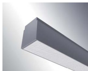
Colourless methacrylate TXT diffuser with outer surface microtextured with micro-pyramids to reduce levels of luminance in the upper angles of emission.
