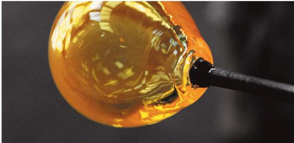
The raw materials react during the melting process and blend into a molten substance which is mixed almost completely and degassed. The glass, liquid like honey, flows through a bottom channel known as the throat, from the melting furnace into the working end, where it cools down to about 1200 °C and becomes viscous. And now the glassmakers can begin their work.
