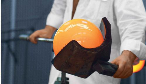
The post maker blows a small amount of air into the blowing iron with his mouth and the raw glass expands, reduces its wall thickness, cools down rapidly to about 600 °C and solidifies. During the cooling period, the blowing iron with its attached glass post is carried by the post carrier to the adjacent opal glass tank. Here the "caser" takes over the blowing iron with the post.
